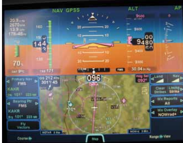
An R9's Integrated Flight Display, installed in an SR22 G2, passing near South Bend, Ind. (KSBN).
