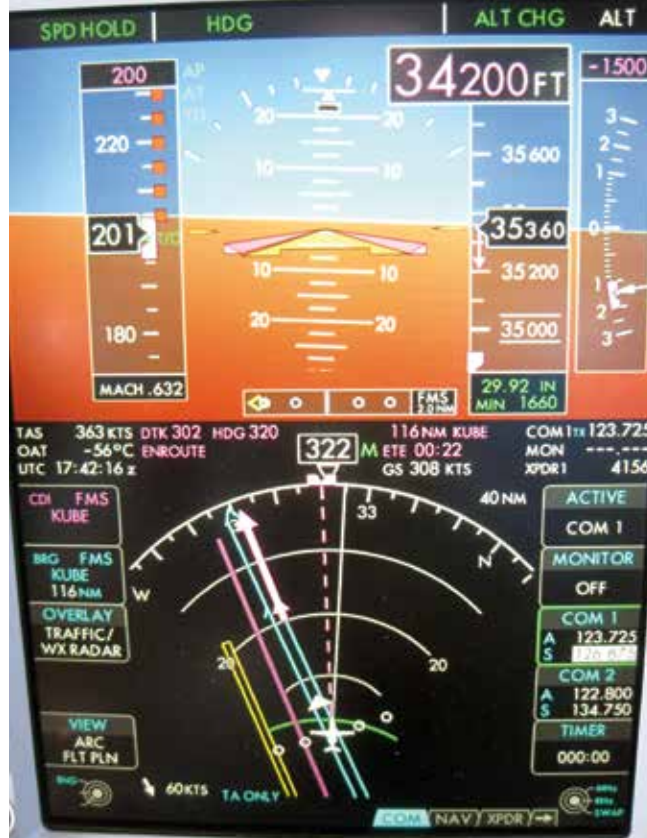
One of the author's favorite features of the PFD is that when something is being adjusted by the pilot, it expands to draw the pilots attention. In this photo, the altitude pre-select is being adjusted, thus its momentary large font.
