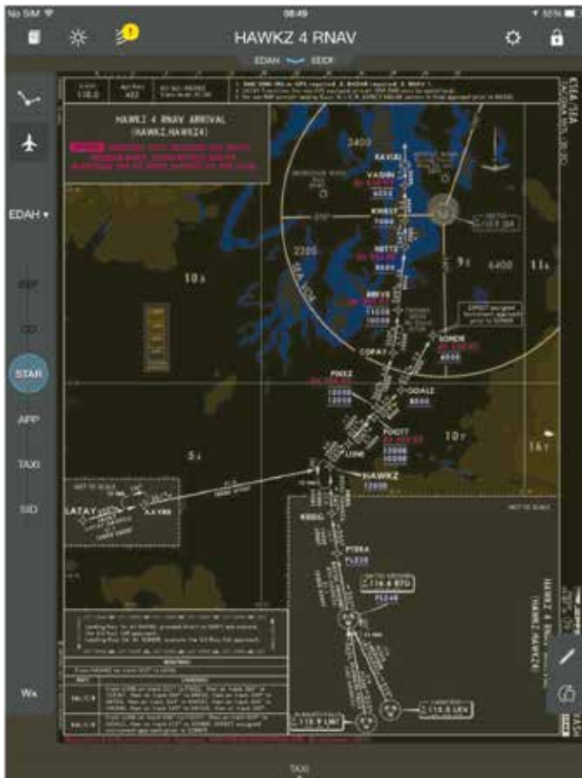
Figure 4: A screen shot of the HAWKZ4 Arrival in “Night Mode.” Note that while the speed restrictions are still displayed in magenta, the normally-magenta MSA sectors become amber. Terrain and water features remain equally obvious in night mode, as does the Contours Intervals scale.
