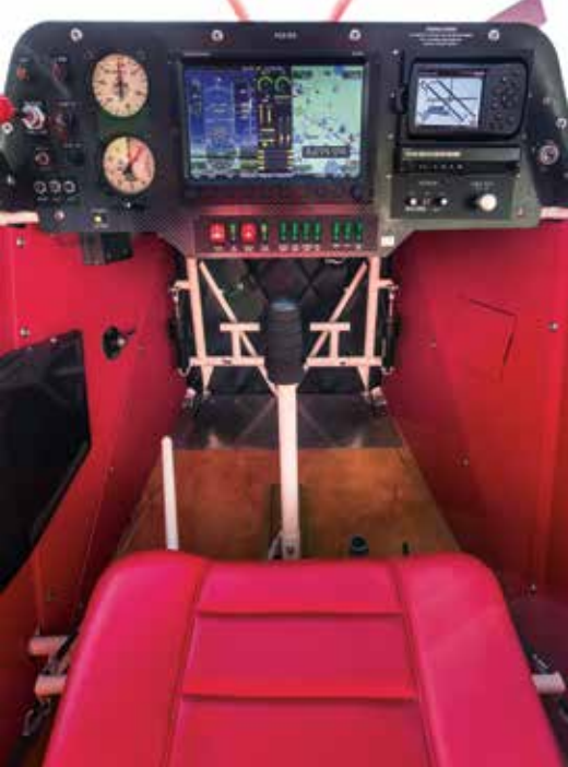
The "Cirrus-ized" panel of the Daytona Cub features carbon fiber structure, large glass displays and an autopilot.
