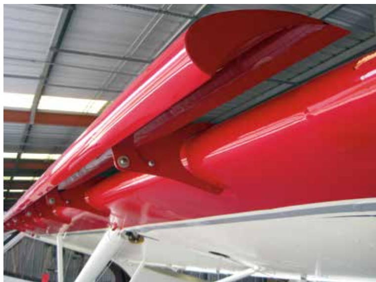
The Cub's leading edge slats, in the fully extended position, help give it uncommonly slow speed flight capabilities
