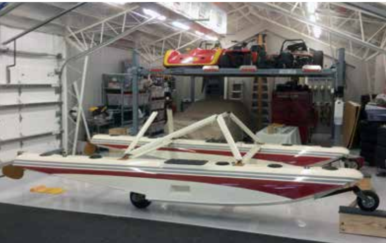
The composite amphibious floats wait patiently in the back of Hein's shop (watched over by some of his prized race cars) for their installation on the Daytona Cub.
