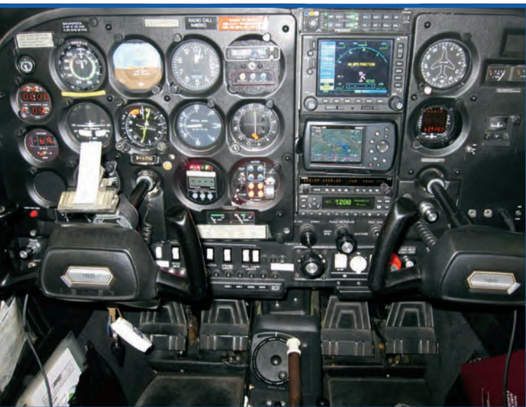
The SkyWagon's updated panel, including WAAS, engine monitoring, XM WX, radar altimeter and a slick gear position warning system that supplements the lights with audible advisories on whether the gear is safe for a water landing or a runway landing.
