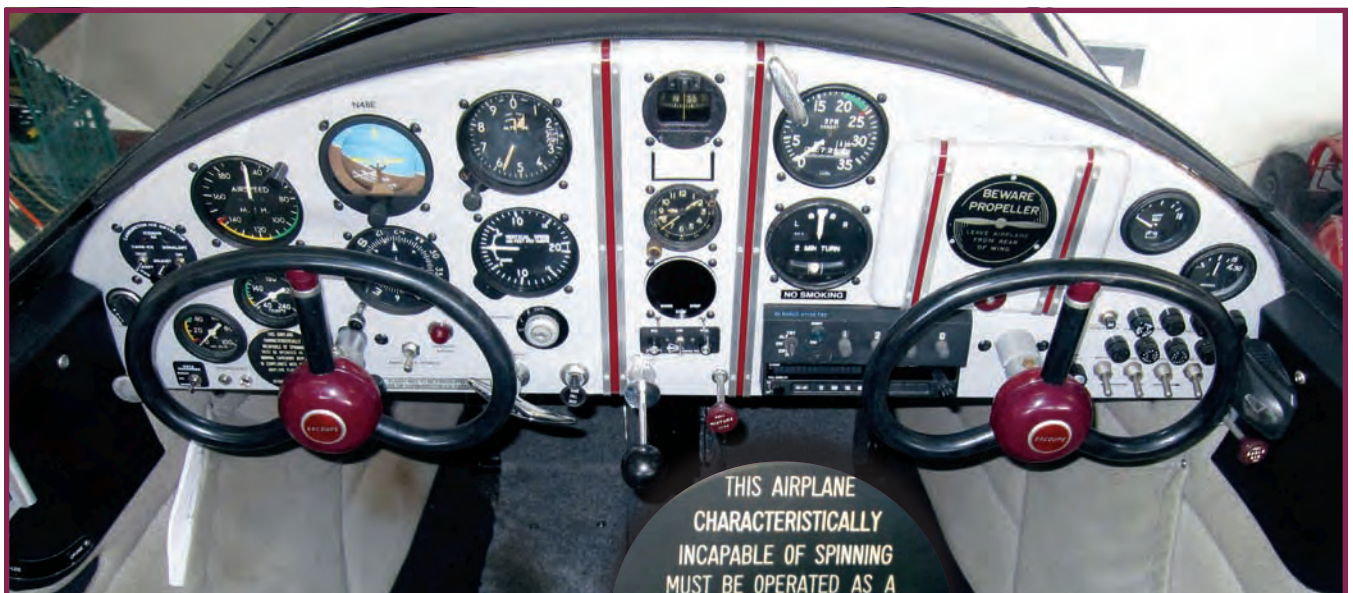
Above, the updated panel of N48E. The carb-ice detector is on the far left, the digital engine analyzer is in the center stack and the original glove box (complete with its cardboard interior) is retained on the right.
