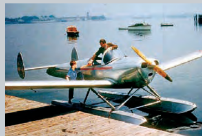
A rare color photo of the Edo float-equipped Ercoupe, most likely a marketing photo. Note the open cockpit.
