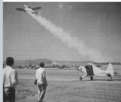
In 1941, the concept of Jet Assisted Takeoff (JATO), also known as Rocket Assisted Takeoff (RATO), was first tested using a military-owned Ercoupe. The Ercoupe (airborne) and the aircraft in the foreground were said to have the same basic takeoff performance (in time and distance required). They began their takeoff rolls together and the photo was snapped just as the lower aircraft broke ground. The picture says 1,000 words about the success of the JATO-assisted performance boost!
