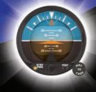
When your panel goes dark or your vacuum system fails, the Lifesaver® powers on – for one full hour. Mid-Continent Instruments is the only company to bring you an electric attitude indicator with a built-in battery backup. With one hour of emergency attitude reference, you have the precious time you need. And its 7,500-hour lifespan is more than double that of most electric gyros – at about two-thirds the cost. Can you live without it? Available from your local avionics retailer.
