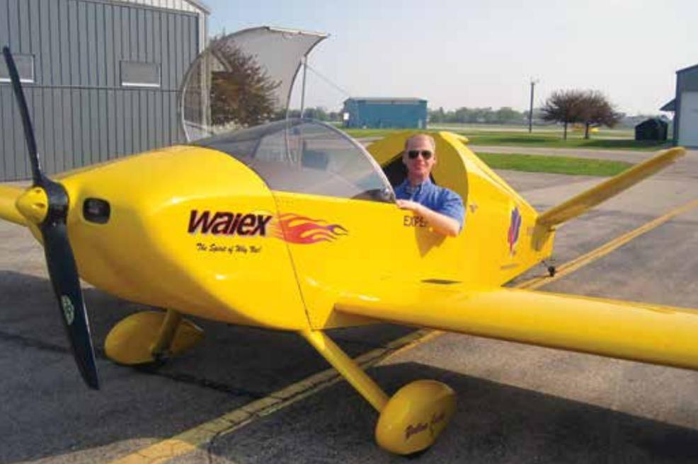
*The author, after checking out in the WaieX. The Y-tail design is purely for aesthetics and offers no performance, handling, or weight advantages/disadvantage over the standard-tailed Sonex designs. However, the WaieX's good looks have proven popular with buyers seeking unique "ramp appeal."*
