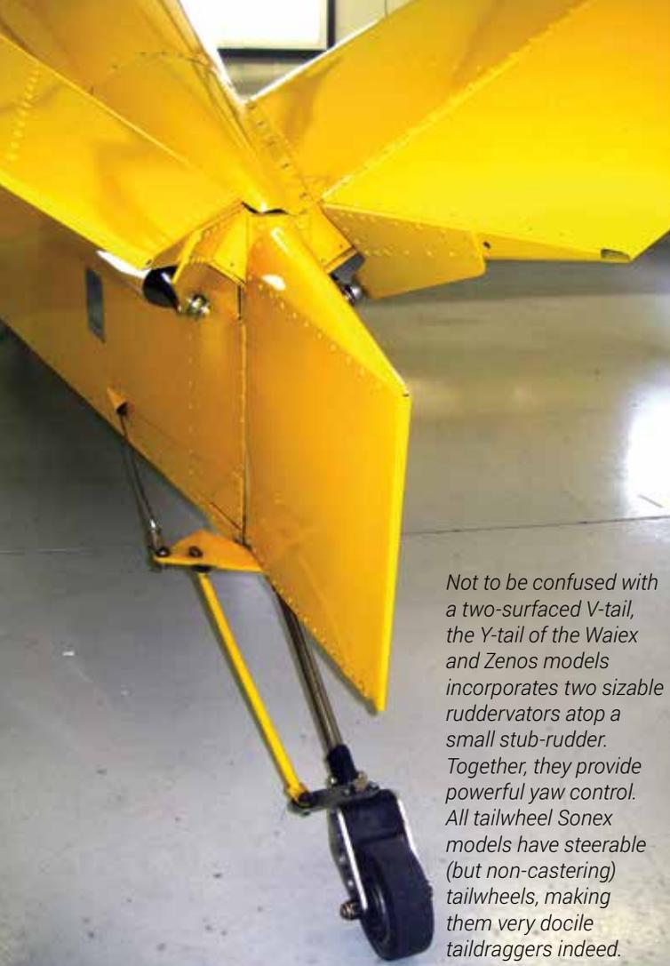
*Not to be confused with a two-surfaced V-tail, the Y-tail of the WaieX and Zenos models incorporates two sizable ruddervators atop a small stub-rudder. Together, they provide powerful yaw control. All tailwheel Sonex models have steerable (but non-castering) tailwheels, making them very docile taildraggers indeed.*
