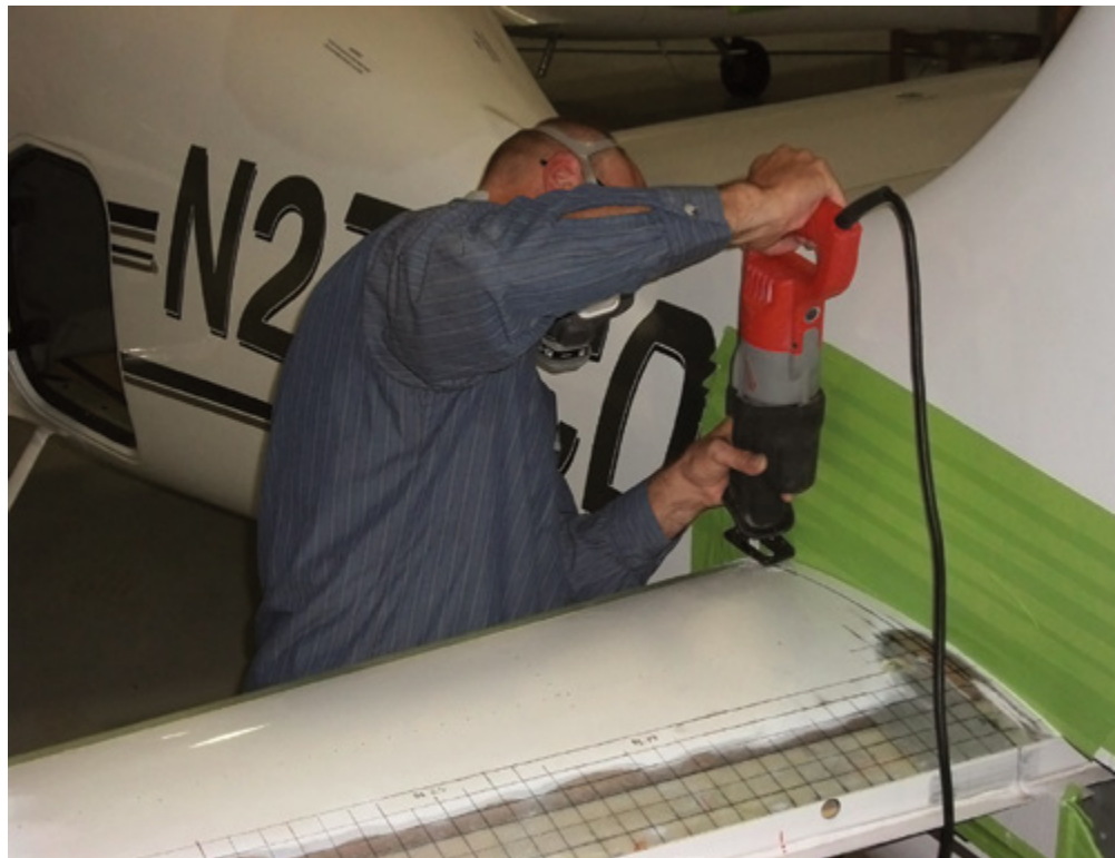
» A Wisconsin Aviation technician uses a Sawzall to cut off the left horizontal stabilizer after the decision was made not to attempt to repair it. Instead, a brand-new horizontal stabilizer, built by Cirrus Aircraft, would be installed.
