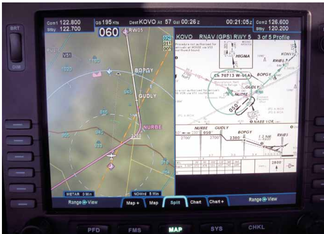
A favorite R9 feature for the author is the split-screen MFD. This is one such option, seeing the traditional moving map and the geo-referenced approach chart simultaneously. Similarly, you could elect to have the flight plan displayed on the right half of the screen. He often uses both options during various phases of instrument approaches.
