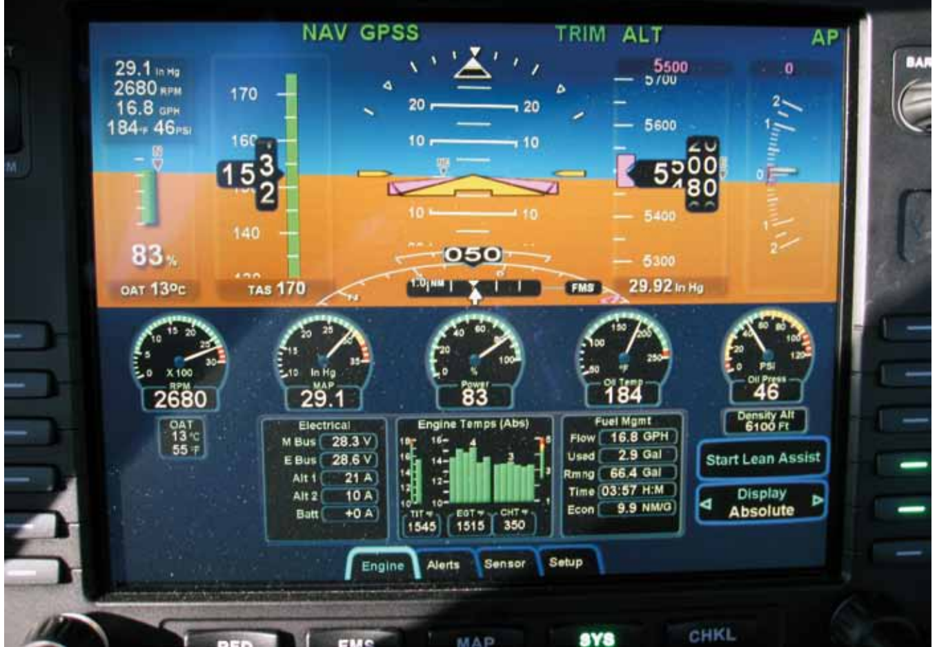
One feature of R9 the author has grown to appreciate is the option of displaying engine data on the PFD. Above is his preferred display convention for takeoff and initial climb (especially when launching into low IMC).
