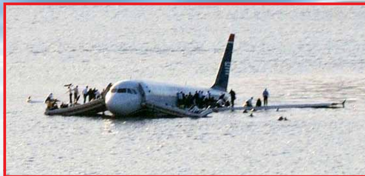
US Air 1549 floats in the Hudson River while passengers begin to egress onto the wing and forward slides (which double as flotation devices). Rescue boats were on the scene almost immediately.
