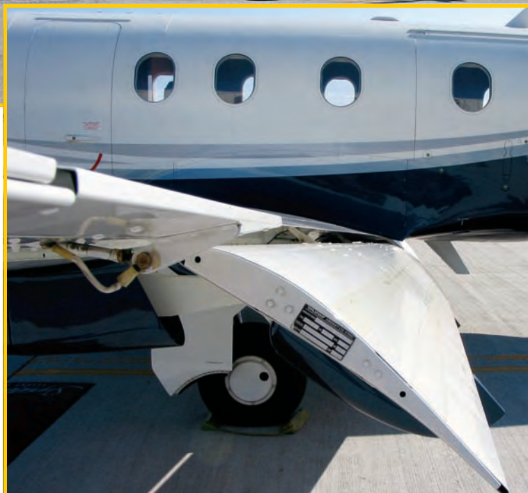
The massive fowler flaps help the PC-12 fly at Cirrus-like approach speeds, in spite of it being three times the weight of a Cirrus.
