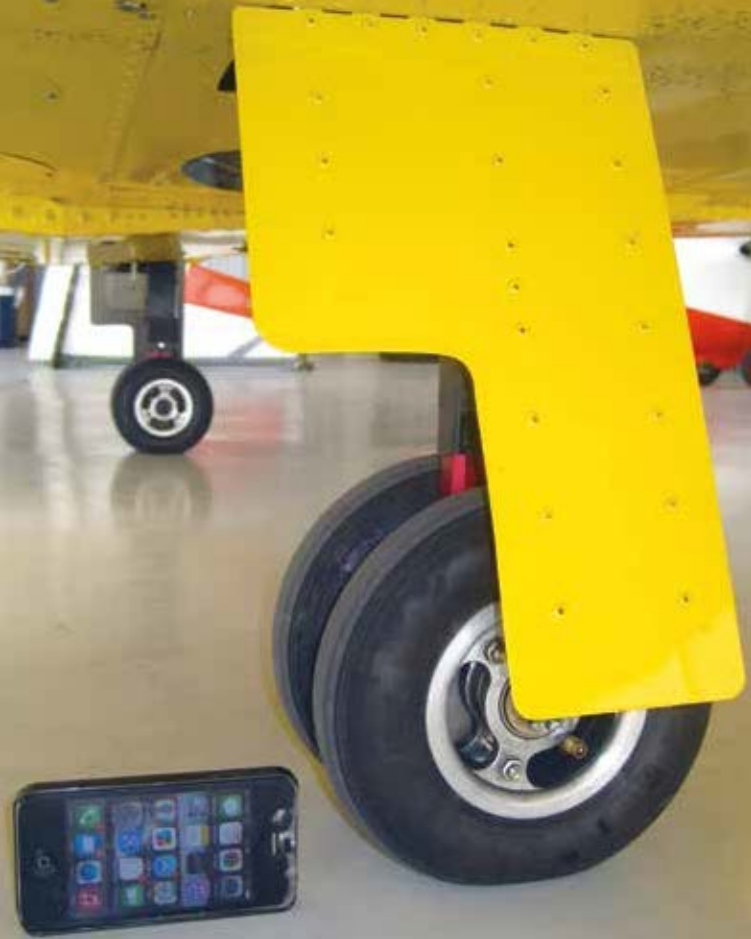
For size perspective, the author placed his iPhone4® next to the SubSonex's main gear. Each tire is inflated to 75 psi and is about the size of a breakfast waffle. Though short-stroked, the struts provide sufficient shock adsorption for landing.
