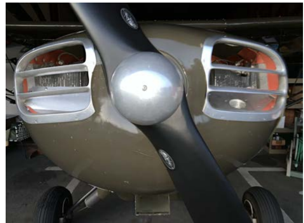
(Left) The original Dataplates for the L-6, inside the cabin. (Right) view of the engine cowling showing the cooling grill adapted from a Stinson. While this is non-standard for an original wartime L-6, the owner chose to employ it for aesthetic reasons. (photos by Matthew McDaniel)
