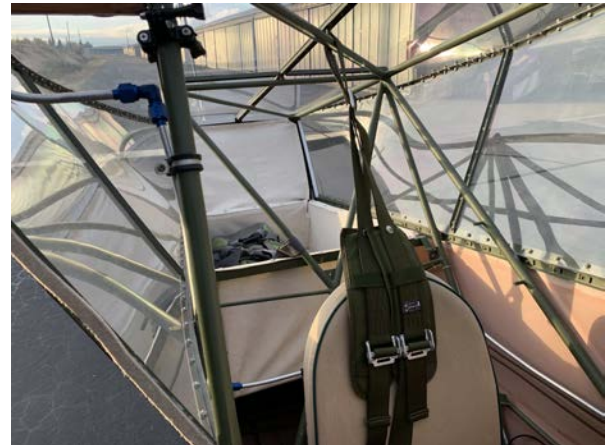
(Left) A view of the L-6 instrument panel, which is mostly stock, except for the modern communications and navigation gear which makes modern flying far safer. (Right) You can get a fair idea of the aircraft's exceptional visibility from this cockpit image, which also reveals the four-point seat harness. While this is not original to the design, which employed a simple lap belt, it is a modern concession to aircrew safety which still has a military feel to it. (photos by Matthew McDaniel)
