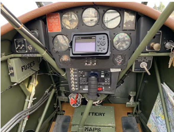
(Left) A view of the L-6 instrument panel, which is mostly stock, except for the modern communications and navigation gear which makes modern flying far safer. (Right) You can get a fair idea of the aircraft's exceptional visibility from this cockpit image, which also reveals the four-point seat harness. While this is not original to the design, which employed a simple lap belt, it is a modern concession to aircrew safety which still has a military feel to it. (photos by Matthew McDaniel)
