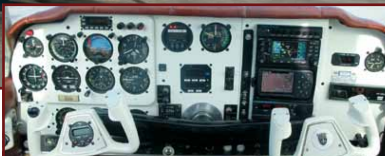
The V-Tail's panel may seem antiquated by Cirrus standards, but it has a WAAS GPS, a fully coupled A/P, and XM weather capabilities.
