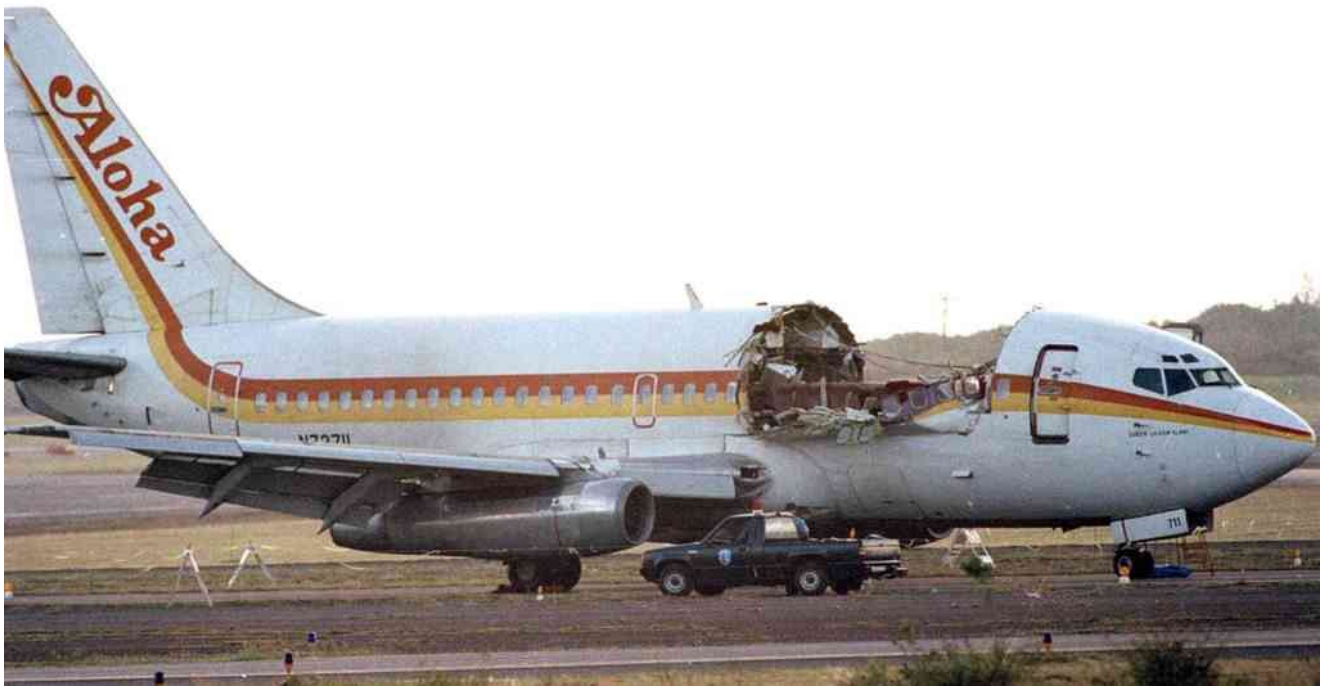
Aloha Airlines Boeing 737 (-200 Series) on the tarmac of Kahului Airport (OGG) in 1988. The major structural failure killed one flight attendant, severely injured several passengers, and caused the flight crew to make an emergency diversion and landing at OGG. [Photo Credit: Wikipedia]
