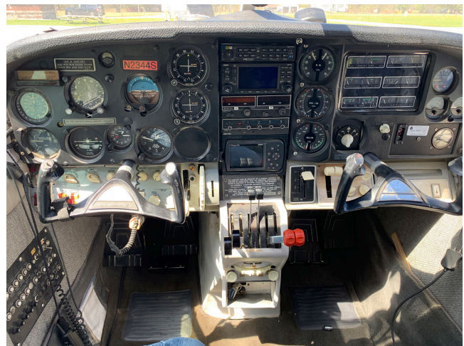
The panel of Anderas' 1965 Skymaster has only been updated in its radio stack (partially) since rescue. The empty slot at the bottom of the power quadrant is where the inoperative autopilot was removed. [Matthew McDaniel]
