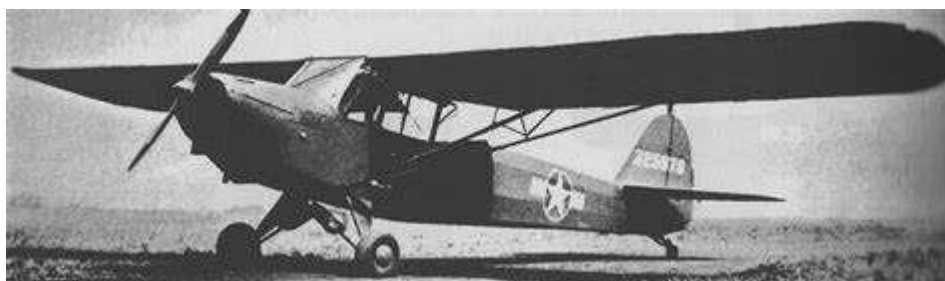
This grainy war-time image of an L-2M can be distinguished from previous L-2 models by its fully enclosed cowling (introduced on the M-model).
