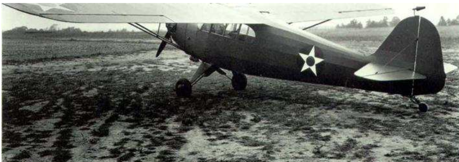
One of four Taylorcraft Model Ds sold to the USAAC, who designated them YO-57, in the autumn of 1941. The production O-57 was later re-designated L-2. Note this pre-production model lacked the full glazed fuselage roof panel between the wings. The O-57/L-2 retained the same tall fuselage of the civilian Model D, while the fuselage was lowered behind the wing in the subsequent O-57A/L-2A models.
