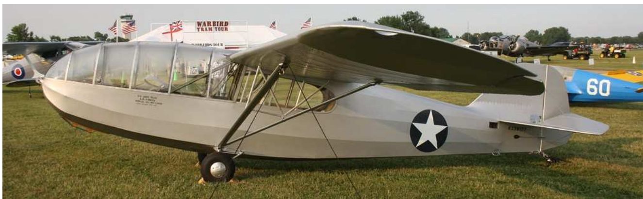
The TG-6 was a 3-seat training glider that developed out of the Taylorcraft L-2. It would also be the first L-2 derivative to utilize wing spoilers. This restored and flyable example is pictured on display at EAA AirVenture in Oshkosh, WI in 2018.
